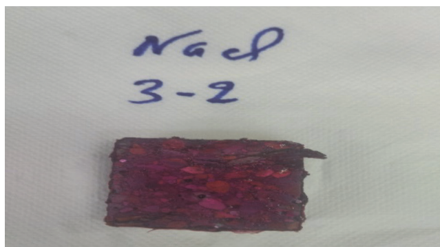
Figure 10. Carbonation test 1 day after extraction from NaCl
