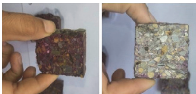
Figure 11. Carbonation test 20 days after extraction from NaCl solution
