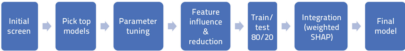
Figure 4. Linear workflow for the development of the Wi-prediction model
