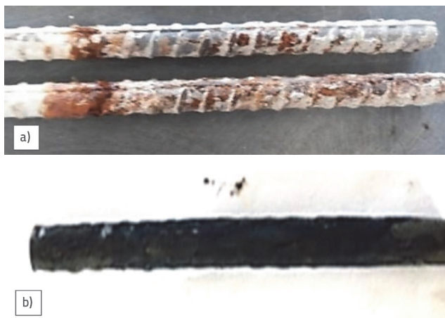
Figure 8. a) Uncoated rod; b) PPE coated rod
