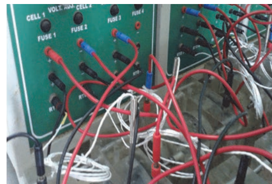
Figure 4. Rapid chloride ion penetration test
